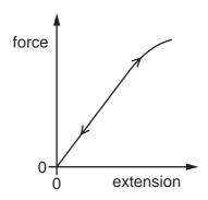
The graph line for the wire being loaded is the same as the graph line for the wire being unloaded.
