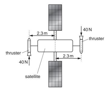
What are the magnitudes of the torque and the resultant force acting on the satellite due to the two thrust forces?
