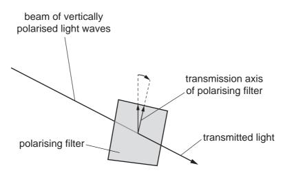
The filter is first rotated clockwise by an angle of  $30^{\circ}$  so that the transmitted light waves have intensity  $I_{30}$ . The filter is then rotated clockwise by a further angle of  $30^{\circ}$ .
